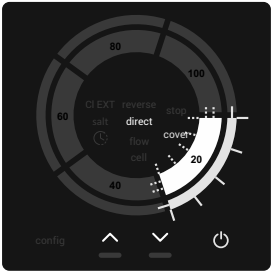
COVER ACTIVATED Led COVER ON Prod 20% fixed, setpoint 20% blinking
