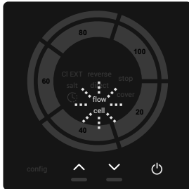
ALARMA FLUJO GAS Leds FLOW & CELL parpadean
