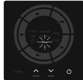
ALARMA FLUJOSTATO Led FLOW parpadea
